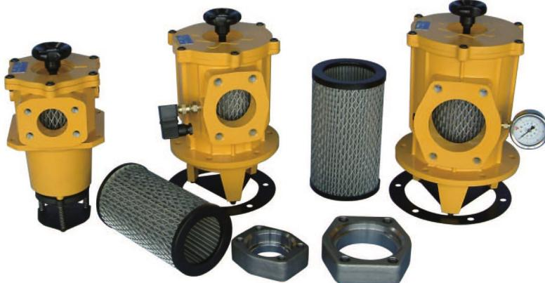
The ST series are suitable for flow rates to 850 l/min and filtration from 25 micron to 250 micron. A major feature of these filters is that the filter element can be changed without emptying the reservoir. The ST series filters are without bypass and include a magnetic prefilter. The filtration flow from inside to outside of the filter element ensures that the contaminant is collected inside the element itself, avoiding contact with tank oil during element change.
